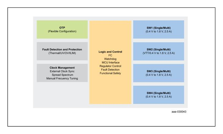
View additional information for Multi-Channel (4) PMIC for Automotive Applications – 4 High Power, Fit for ASIL B Safety Level.
