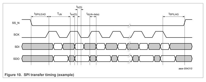
An example SPI timing diagram is shown in <u>Figure 10</u>. Data is captured on the falling edge of the clock and transmitted on the rising edge. Both master and slave must operate in the same mode.
