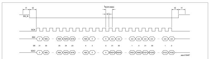
t3: The SPI clock signal (SCK) must be stable for at least half a clock period (t<sub>SPIDV</sub>) between the reception of longword[0] on the SDI input and the transmission of longword[1] on the SDO output.
